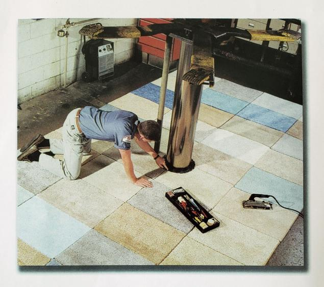
Forty carpet samples, representing a wide range of fibers, construction and design, were used to carpet the grease bay in a busy Union 76 service station.
